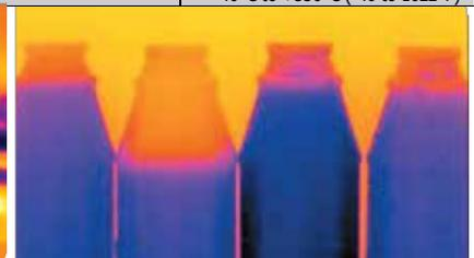
Detecting liquid level in visually opaque bottles
